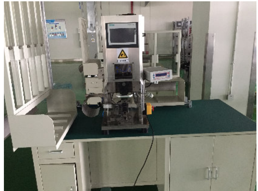
Terminal Crimping machine Punching pressure: 6T
