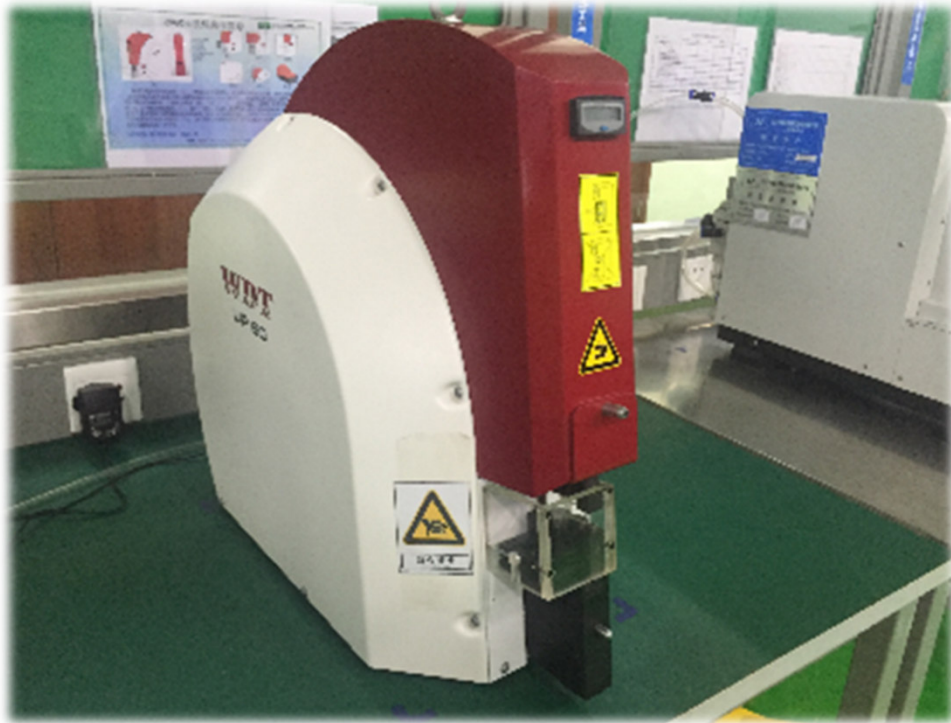
Crimping machine WDT(Swiss) Range:6mm 2 -300mm 2
