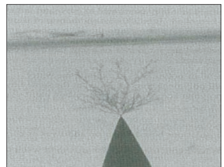
Fig. 6: An electrical tree in epoxy resin [1].
